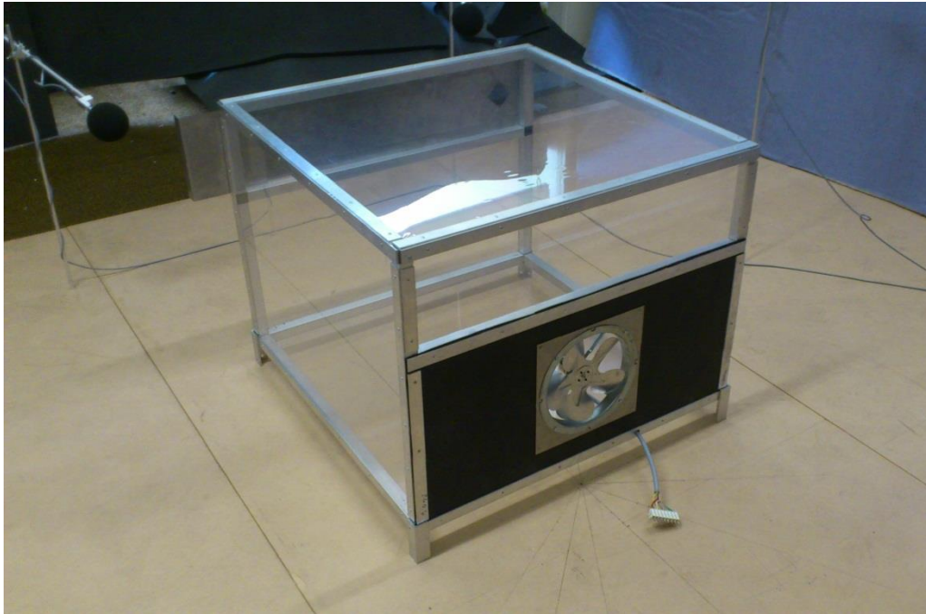
Plenum test chamber
