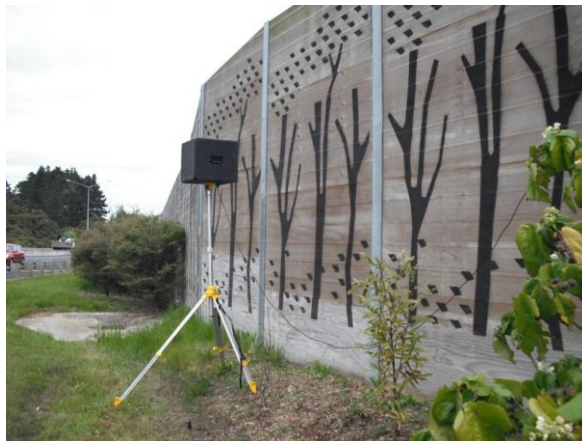
Noise source (left) and microphone array (right) set up for measurement
