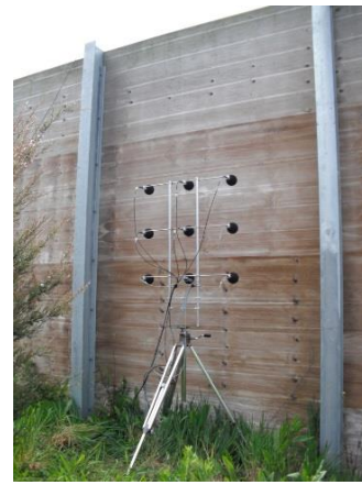
Noise source (left) and microphone array (right) set up for measurement
