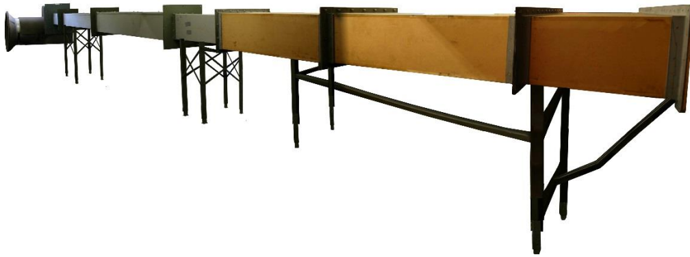
Duct Noise Test Rig
