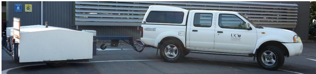
Tyre road noise measurement trailer and towing vehicle
